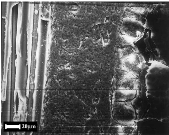
Fig. 4. SEM cross-section of SiC f /SiC composite after 10000 h of exposure in Li 4 SiO 4 .
